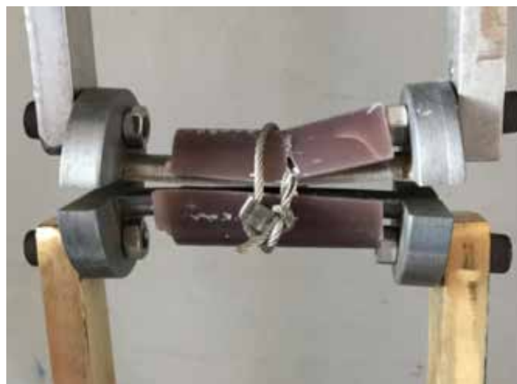
Figure 3. Failure of the system: breakage of upper saw bone fragment.
